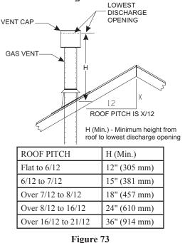
Note that for steep roof pitches, the vent height must be increased. In high wind conditions, nearby trees, adjoining roof lines, steep pitched roofs, and other similar factors can result in poor draft, or down-drafting. In these cases, increasing the vent height may solve this problem.
